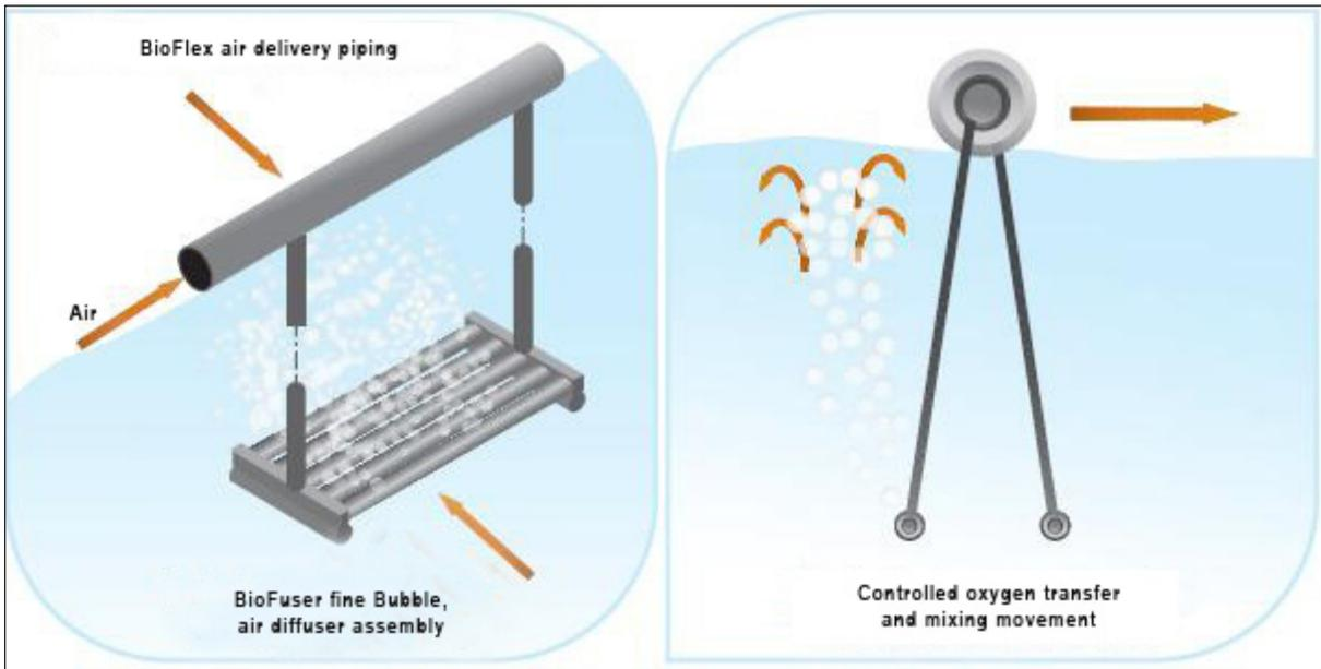
Figure 2: Fine Bubble Diffuser Mechanism
