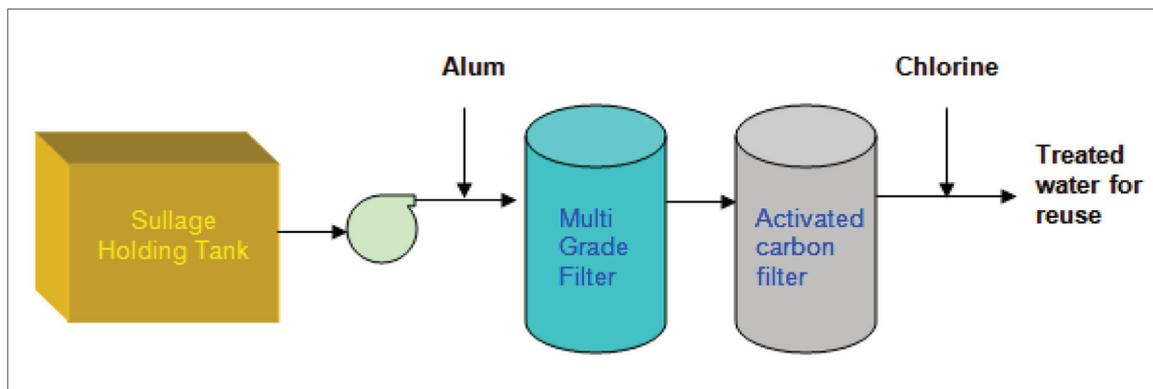
Figure 2: Sullage Recycle System
